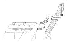
9.3 To protect against mechanical damage, protection pipes no. 716X or no. 718X are recommended for the exterior wall duct.
